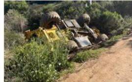
SSI - In April 2024, a Reach Lift traveling over narrow roadway rolled down embankment causing injury to operator and in patient hospitalization. (SDGE)
